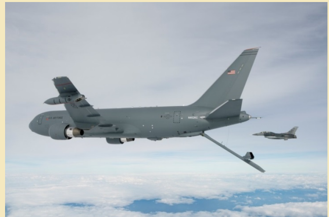
The KC-46A Pegasus Tanker deploys the centerline boom for the first time. The boom is the fastest way to refuel aircraft at 1,200 gallons per minute. (Boeing photo by John D. Parker)
